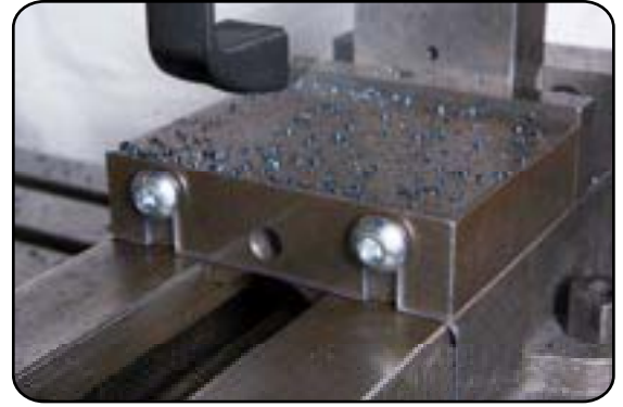
Two 1/2"-13 x 1" button-head cap screws holding the shield to the vise.
